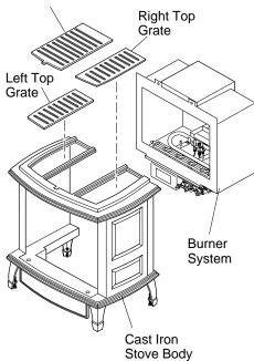
Figure 15 - Installing Burner System Into Cast Iron Stove Body
